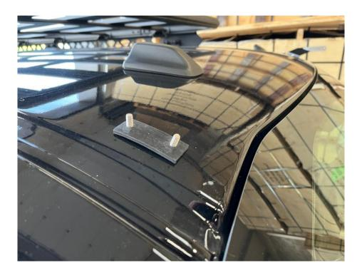
Lightbar bracket & mounting bracket can now be installed onto van roof.
