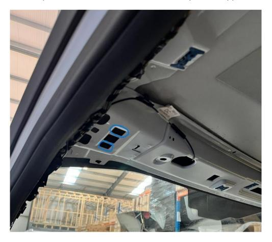
Drill a 6mm hole through the van roof, in the centre on the square hole shown below.
