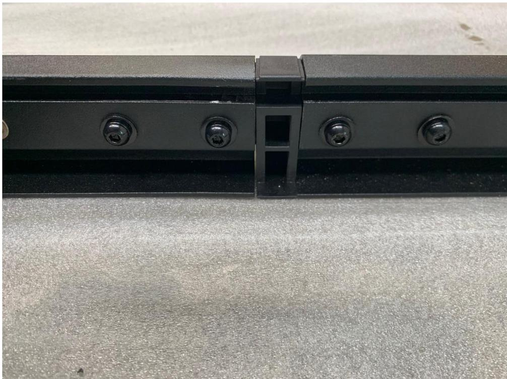
**Step 10** - Align holes in the cross-section support rails with the T-slot bolts previously fitted to long support rails, ensure the channel recess, and threaded inserts are facing upwards, (below image).
